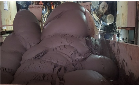
图1 渣土现场取样 Fig. 1 On-site sampling of spoils
