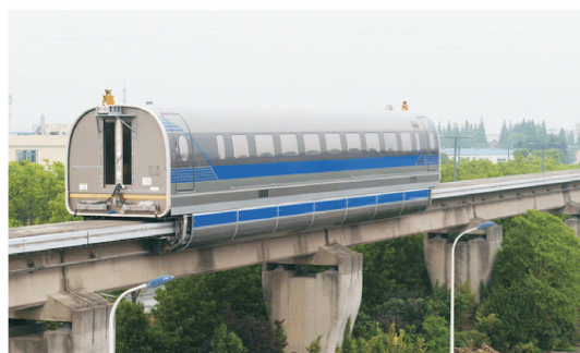
图 14 同济大学 600 \text{ km} \cdot \text{h}^{-1} 高速磁悬浮试验样车 Fig. 14 High-speed maglev test sample vehicle with speed of 600 \text{ km} \cdot \text{h}^{-1} in Tongji University
